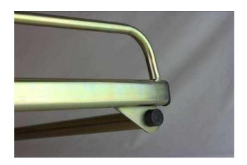
...and fit the roller at the back as you install the other side. The bearings are made from self-lubricating Nylotron (graphite impregnated nylon) and need no additional lubrication. Lastly, you can drop your middle bar into place as well.
