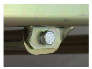
Put one longitudinal in place with the barest nip on the bolts- this will begin to align the cross bars...
