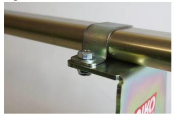
Again, the longitudinal bars are very straightforward- they bolt into the ends of the cross bars with an M8 x 16 bolt with a spring washer.
